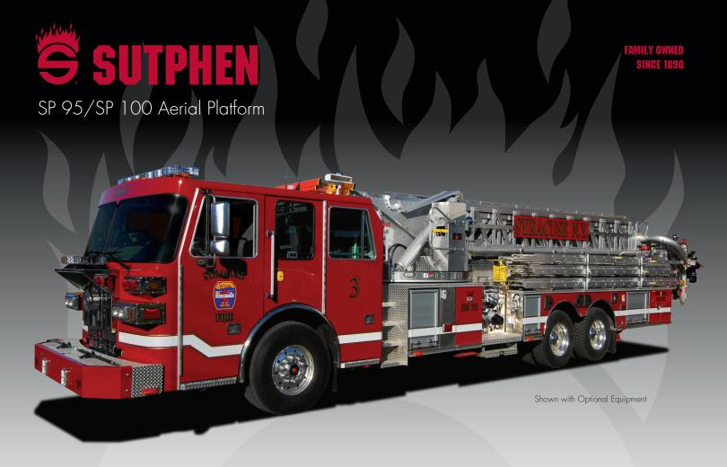
The Sutphen original mid-mount aerial platform design provides unsurpassed safety, performance, reliability, and maneuverability. The mid-mount design allows for lower center of gravity and low profile. The need for only one out and down stabilizing jack on each side provides the industry's quickest and most compact set up.
